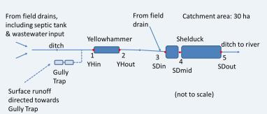
Figure 1. Flow pathways and sampling points at Whinton Hill.
