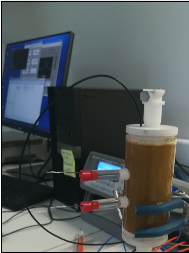
Figure 2. Laboratory set-up that allowed us to explore the electrical signature of the reference soil sampled from CHAR observatory fieldsite
