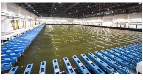
**Experimental Modelling and** Validation of the Computational Modelling for TALOS WEC
