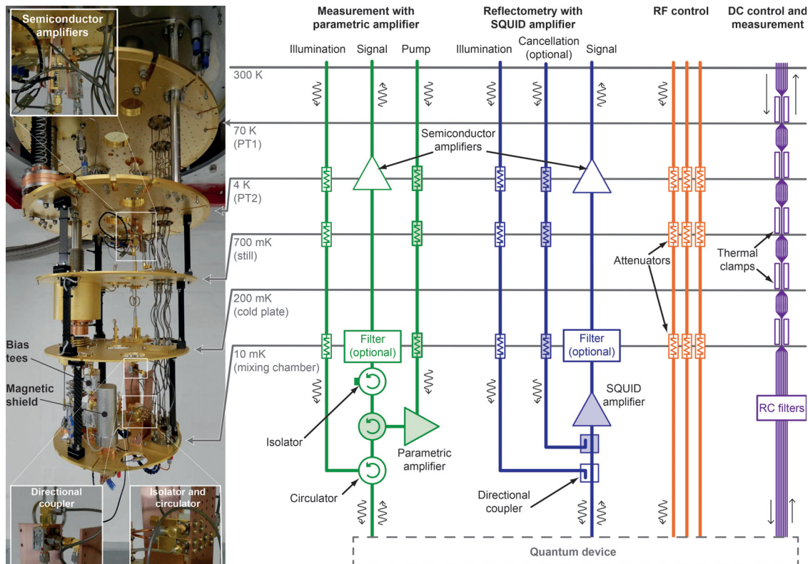
FIG. 31. Right: Typical refrigerator wiring for high-frequency measurements. This setup includes (left to right): Measurement chain using reflection-mode parametric amplifier (based on Refs. 199 and 331); measurement chain using SQUID amplifier (based on Ref. 197); high-frequency control lines using coaxial cable; quasi-dc control and measurement lines using cryogenic loom. Such a setup can also be operated without superconducting amplifiers by omitting the shaded components. To protect the quantum device from thermal radiation, all lines are attenuated and/or filtered at various stages inside the refrigerator, and thermally clamped to minimize the heat load on the mixing chamber. Components drawn below the 10 mK line are in thermal contact with the mixing chamber plate but not necessarily below it. Left: A Triton 200 refrigerator wired in a similar arrangement. This refrigerator is equipped with a flux-pumped parametric amplifier 203 and therefore contains two bias tees (not drawn in the circuit diagram) through which the amplifier is biased. Selected components are labeled.
