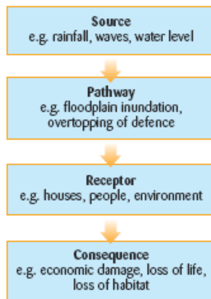
Figure 1.2: The simple conceptual S-P-R-C Model for representing the systems and processes that lead to flood consequences. Source: FLOODsite (2007)
