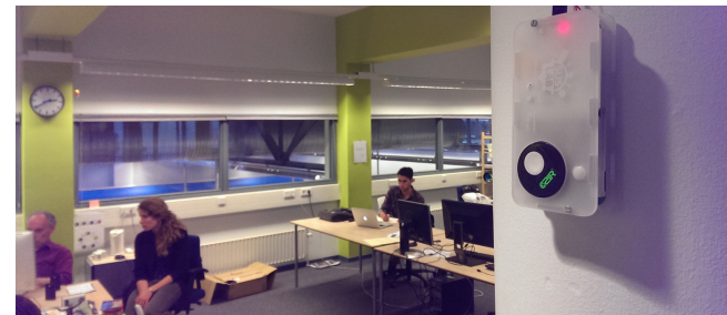
Figure 1. Wireless sensor node for measuring office comfort.
